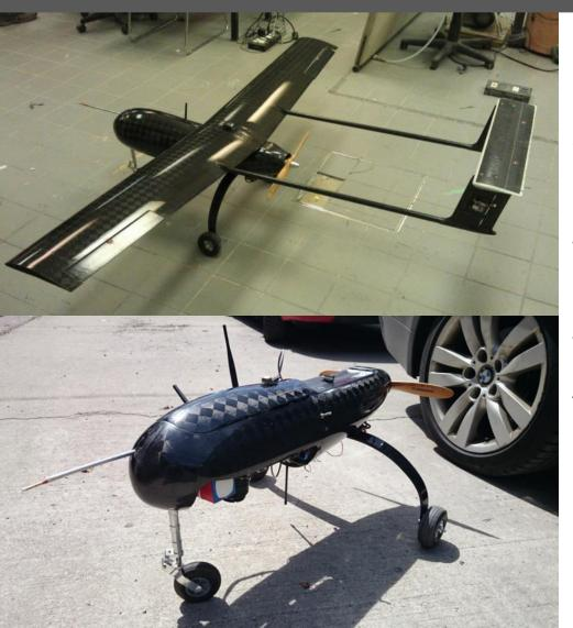
Pusher-style AC with electric powerhouse
